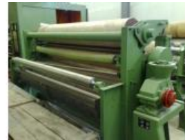
Reference: M-1002 Squeezing and finishing padder Year: 1988 Brand: Artos Width: 2200
