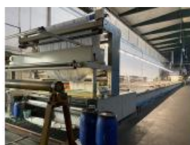
Reference: STV-002 FLAT BED PRINTING MACHINE 9 co... Year: 1995 Brand: Reggiani Width: 3200mm WW
