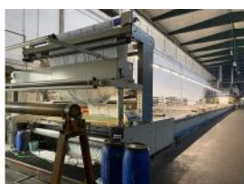
Reference: STV-002 FLAT BED PRINTING MACHINE 9 co... Year: 1995 Brand: Reggiani Width: 3200mm WW
